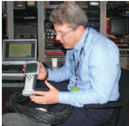
time-domain reflectometer to determine the return-loss of a hank of co-axial cable. He gave a good explanation of how digital audio is transferred along with the picture information, and showed how compressing multi-channel audio into one AES/EBU pair is becoming a very popular technique.
